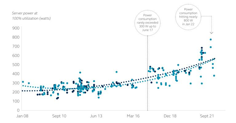
The data shows the sustained maximum power consumption of two-socket servers when running the SPECpower\_ssj2008, which simulates a Javabased business logic. Results for 1U and 2U form factors. Data as at June 27, 2022.
